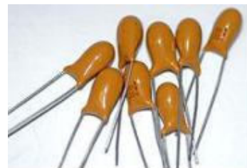
Solid-body, resin-dipped 10 \mu\text{F} 35 V Tantalum capacitors.
