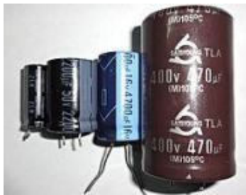
Electrolytic capacitors of different voltages and capacitance
